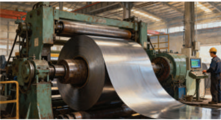
Uncoiling of steel coils
